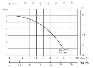
Note: Flow curve information based on 220V/50Hz motor.
